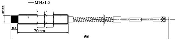
Sensor for PPT-110 version with 9m extension cable
