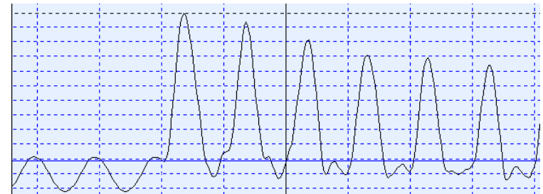
Inrush current captured in waveform mode (32, 16 or 8 samples/cycle)
